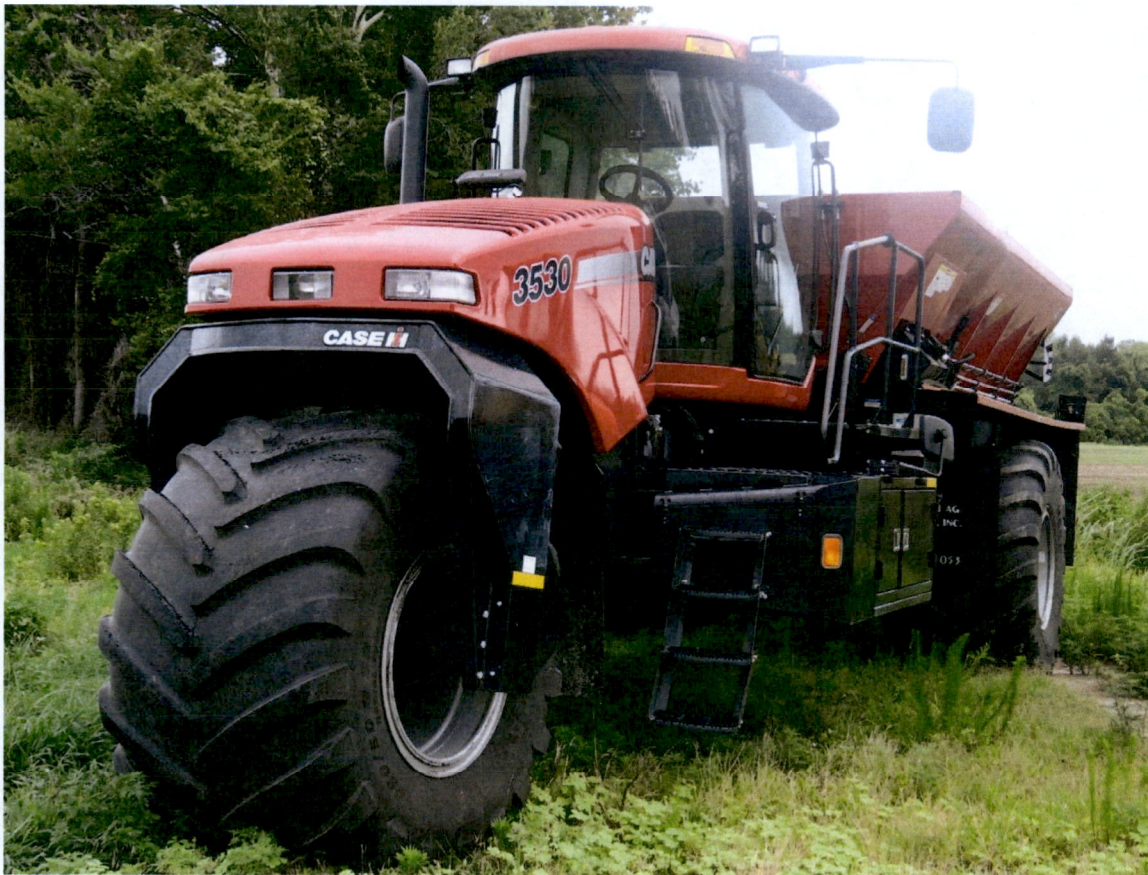
Fig. 12-2. Example of spreader typically used for mill by-products. The spreader shown is a Case.
